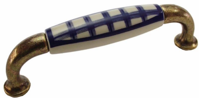
Ref. 640 Tirador ABS / ZAMAK 110 x 32 x 16 mm 96 mm entre taladros
